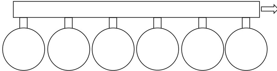
**Figure 3 – Engine Exhaust Manifold (6 Cylinder)**
