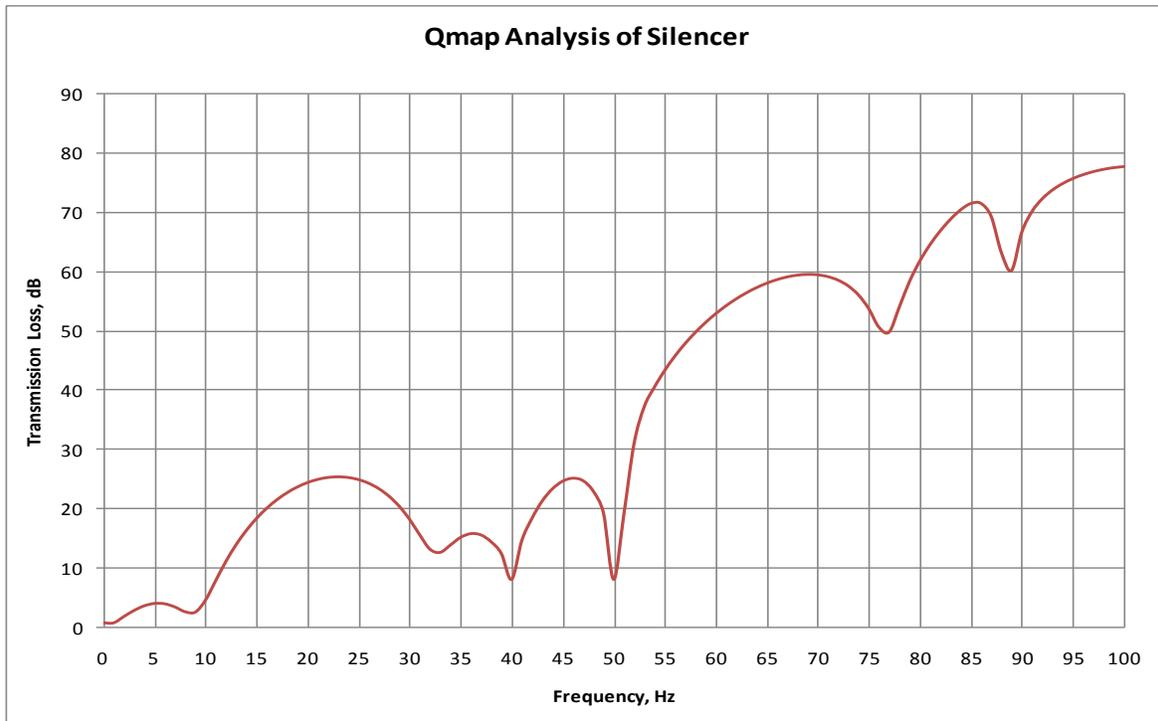
Figure 2 – Analysis of a Three-Chamber Reactive Silencer
